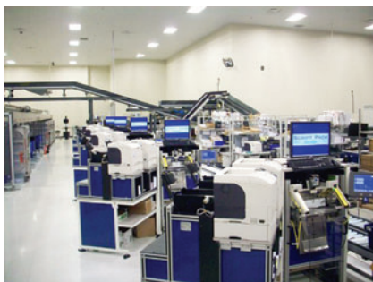
Automated Packaging Systems Inc. integrated an Autobag AB 180 bagging system with proprietary pharmacy fulfillment software developed by R/X Automation to provide a customer solution.
