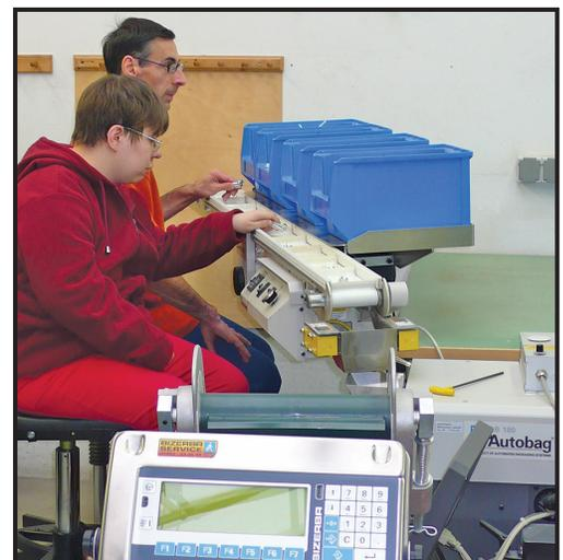
In Glauchau, four different product specific pouch formats are used depending on the number and volume of products to be packaged. Switching the pouch format with Autobag bags-on-a-roll just requires a short series of simple hand movements.
