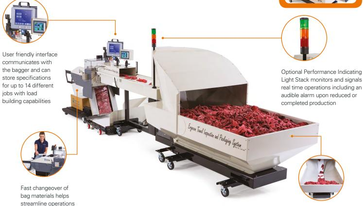
Load bin is just 34 inches high for easy loading with a sling, standard lift table, or by hand
