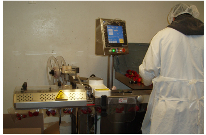
Single-serve portions of fruits and vegetables are bagged by the machine. The unit also has an ink-jet imprinter.
