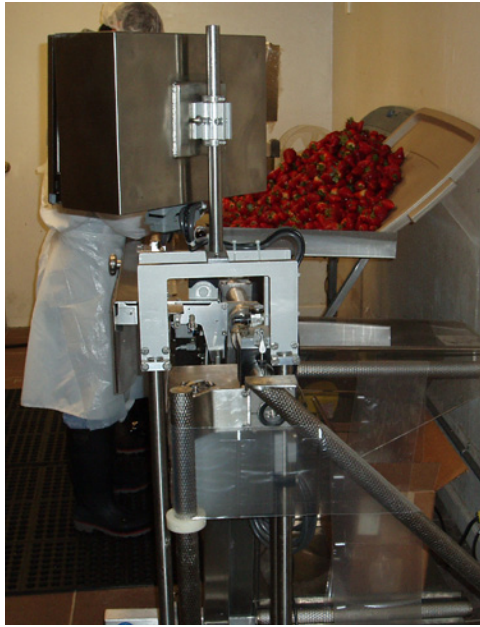
Recently commercialized, the new bagger, above, facilitates single-serve bagging of whole strawberries. It saves time and money, according to Fresno Produce, is easy to set up, clean and maintain, and now packs about 30,000 bags a day for next-day delivery.
