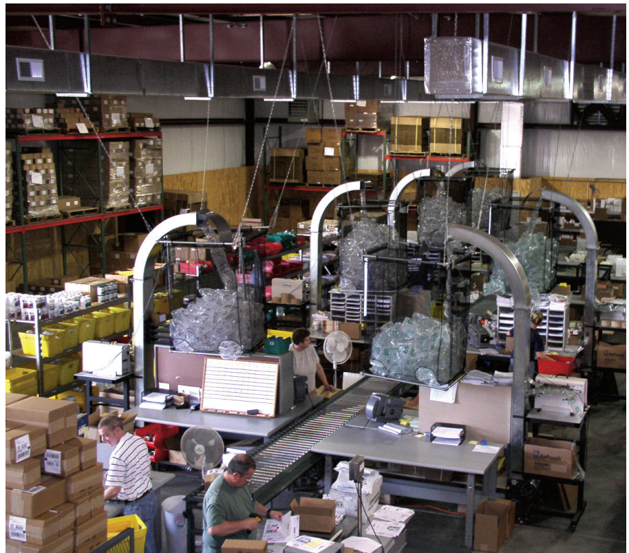
CUSTOM FEED. Automated packing stations move the air pillows from the machine via an air tower into an overhead hopper.
