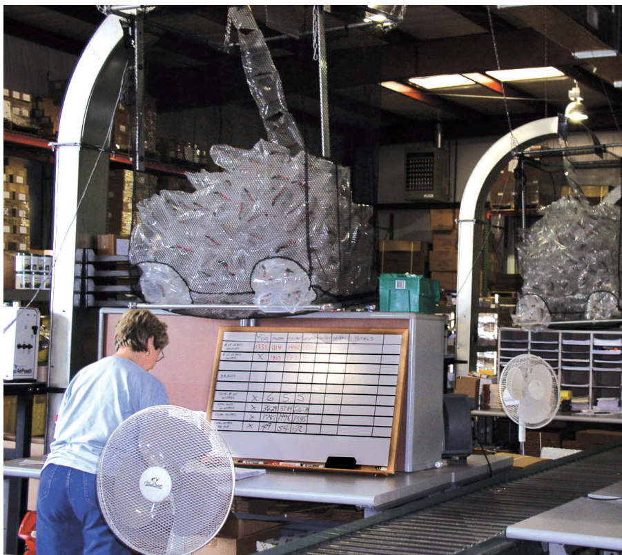
DOUBLE DUTY. Each hopper features two openings to serve two packing stations. Operators can pull lengths of air pillows directly into the packing area, easily tearing off as many pillows as they need.
