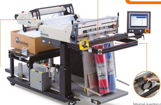
Minimal guarding provides unobstructed access to the open bag
