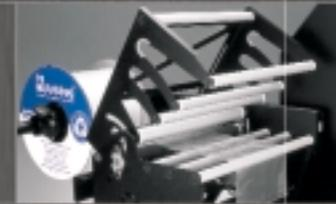
Opposing friction belt design traps the bag web to maintain a constant position for precise product loading and accurate sealing.
